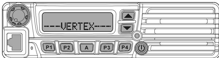
The **VX-4200** Series are full-featured FM transceiver designed for flexible mobile and base station business communications in the VHF or UHF Land Mobile bands. These transceiver are designed for reliable business communications in a wide variety of applications with a wide range of operating capability provided by their leading-edge design.
