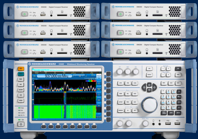
Multiple R&S®EM200 receivers can be operated together with the R&S®ESME wideband monitoring receiver
