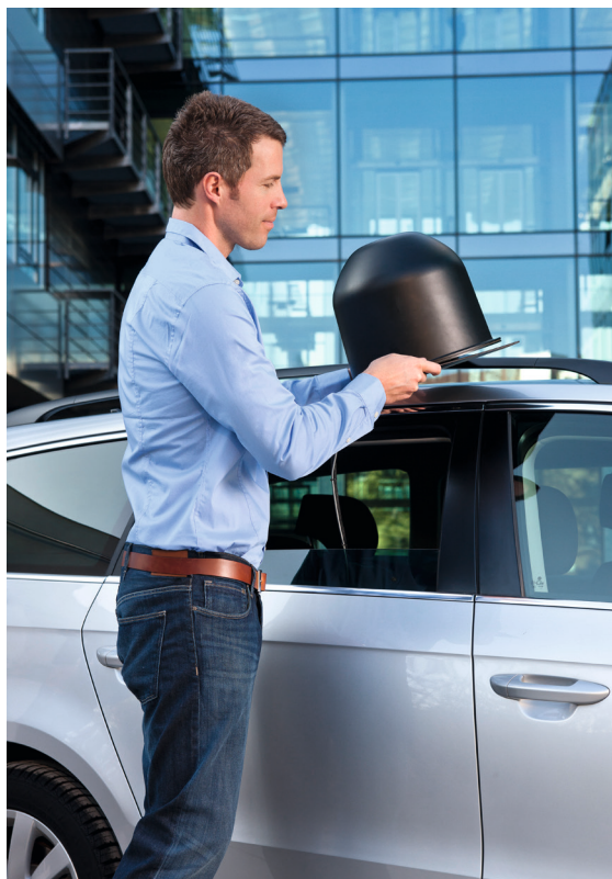
Temporary installation of an R&S®DDF1555 DF system in a commercial vehicle.
