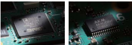
<DSP unit> ADSP-21369 Internal clock speed: 333MHz 32-bit floating point DSP Max. performance: 2000MFLOPS <AD/DA converter> AK4620 ADC Signal/(Noise+Distortion): 100dB ADC Dynamic range, S/N: 113dB DAC Signal/(Noise+Distortion): 97dB DAC Dynamic range, S/N: 115dB
